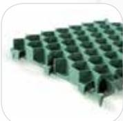
**PRATO SVELTO** is the technical solution for ground consolidation. It is a grass paving system that enables water drainage and is suitable for vehicles. Ideal for building car parks, cycle paths, walkways and green areas. Durable and easy to install, made in HD-PE, it measures 40 x 40 x 4.8 cm. The star cap accessory enables to mark off parking areas or other places.
