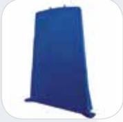
**TELESTOP** is a modular system to be used with TOP 4S, consisting of a stopper and a telescopic extension made of polypropylene that closes the formwork and allows the simultaneous laying of the slab and foundation beams thereby reducing costs. It can be used as a simple stopper or as an extension to avoid cutting the formwork and thereby reducing the laying time.
