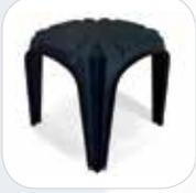
**MAGNUM** is disposable formwork (71x71 cm) made from recycled polypropylene suitable to create ventilated crawl spaces, cavities, floors in any construction or renovation project. It is durable, easy and fast to install (2 pcs / m<sup>2</sup>). It is produced in the following heights: 60 - 65 - 70 - 75 cm.
