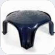
**TOP 4S** is a disposable formwork (50x50 cm) made from recycled polypropylene suitable to create ventilated crawl spaces, cavities, floors and roofs in any construction or renovation project. TOP 4S is made in the following heights: 4.5 - 8 - 13 - 16 - 20 - 25 - 27 - 30 - 35 - 40 - 45 - 50 - 55 cm.
